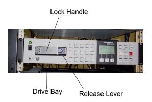
STEP 3: Press the Lock Handle flush with the chassis face to lock the drive in place.
